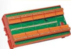
The REM I/O module displays the status of each sensor cell of the MD scanner. Each cell present in the scanner is associated to one L.E.D. on the REM I/O module to display its status. The REM I/O module has a maximum of 64 NPN outputs for connection to a PLC (Programmable Logic controller).
